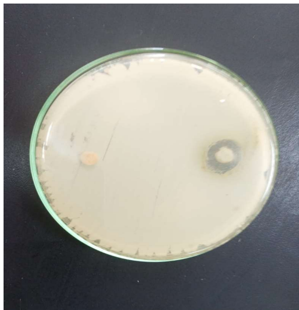
Figure 3 The agar diffusion test showed a zone of inhibition around the specimen disc containing 30% (CuO)-containing PGF (group E on the right) versus control (group A on the left)
