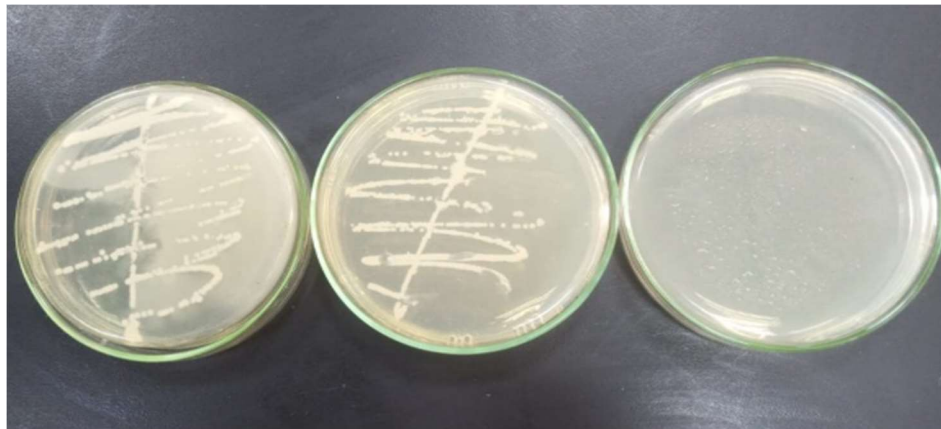
Figure 2 Reduction of bacterial growth on Muller Hinton agar plates with increased concentration of (CuO)-containing PGF (culture from broth containing test specimens group B on the left, group C on the middle and group E on the right, inoculated with S. aureus )
