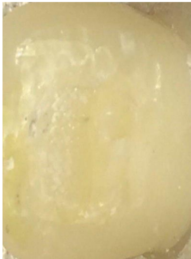
Figure 3 50% to 90% of the adhesive materials remains on the samples' surface.
