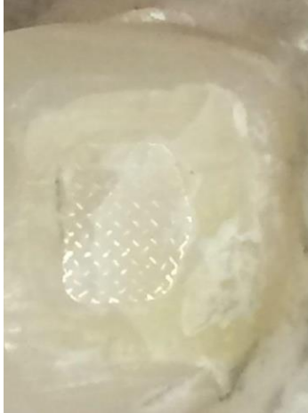
Figure 2 90% of the adhesive materials remains on the samples' surface.
