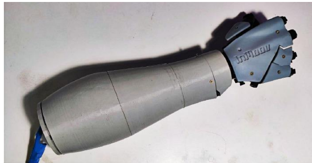
Figure 6 Assembled Prototype of An Anthropomorphic Gripping Device
