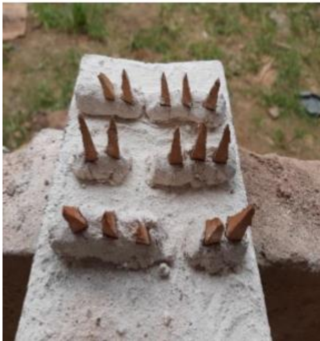
Plate 2 Clay Samples after firing (0-15 wt. % snail shell)
