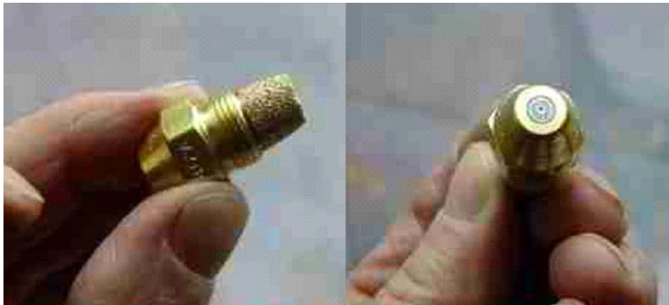
Figure 6 Fuel burner nozzles selected
