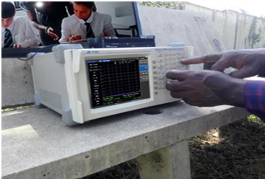
Figure 3 Connection of E8000 A series Spectrum Analyzer to the Receiving Antenna.
