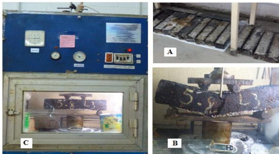
Figure 1. (A) part of the prepared specimens. (B) Failure mode. (C) PRLS Apparatus
