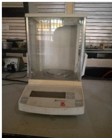
Plate 2: laboratory-type digital balance with 0.01-g precision
