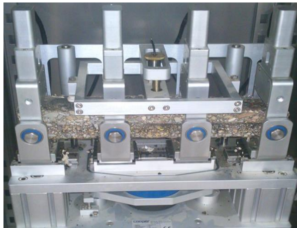
Figure 2. Four-points flexural bending test setup.
