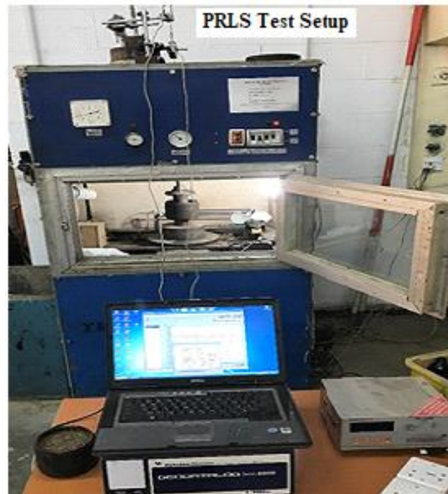
Figure 2. Resilient Modulus Testing at PRLS
