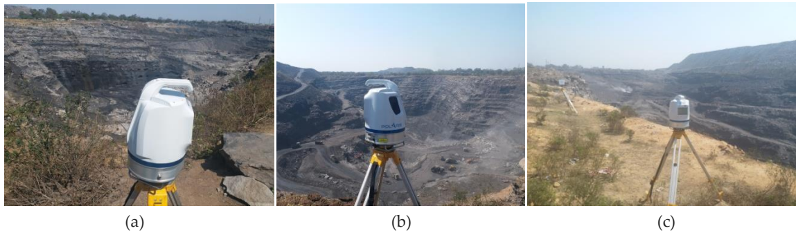
Fig. 2: 3D scanning by TLS at different location
