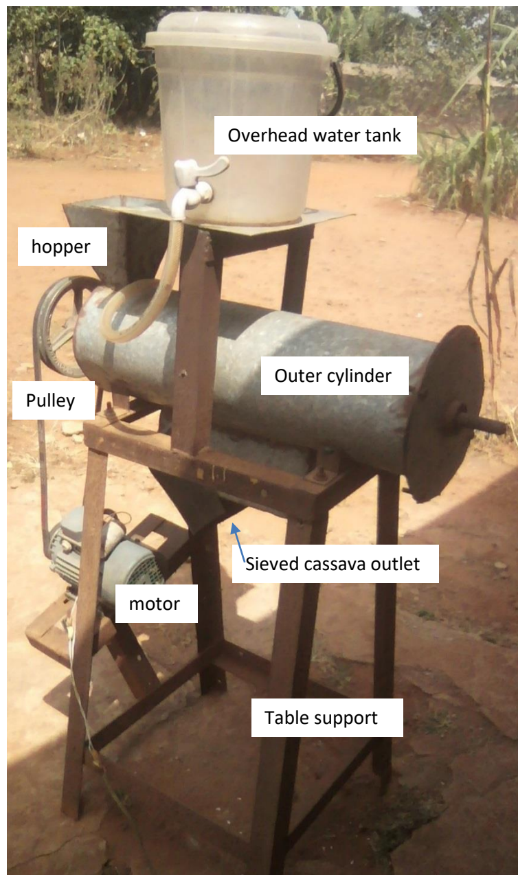
Fig. 5 Completely assembled fermented cassava wet sieving machine
