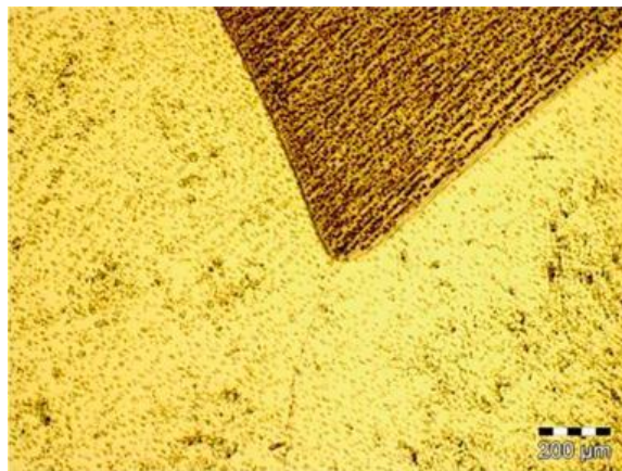
Fig.5. Undissolved tantalum fragment in the FeTaNbTiZrMo alloy.
