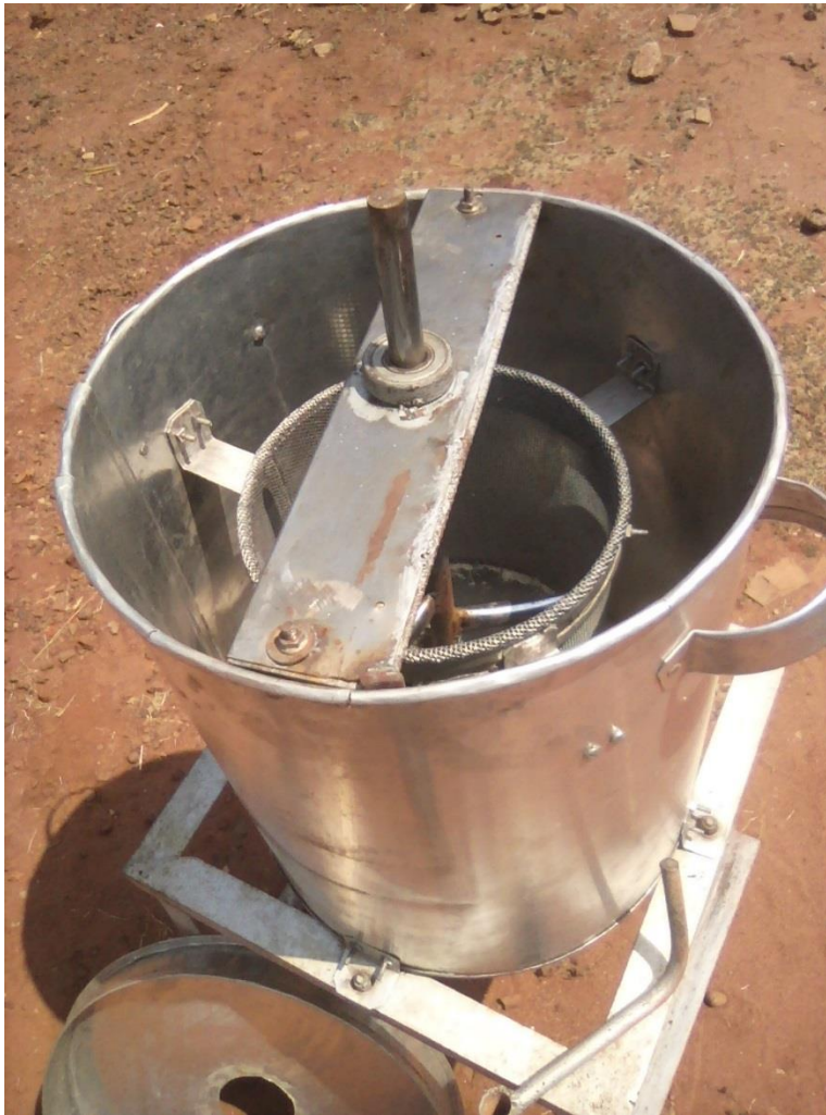
Fig. 2 shows the wet sieving equipment in a ready position to receive fermented cassava pulps
