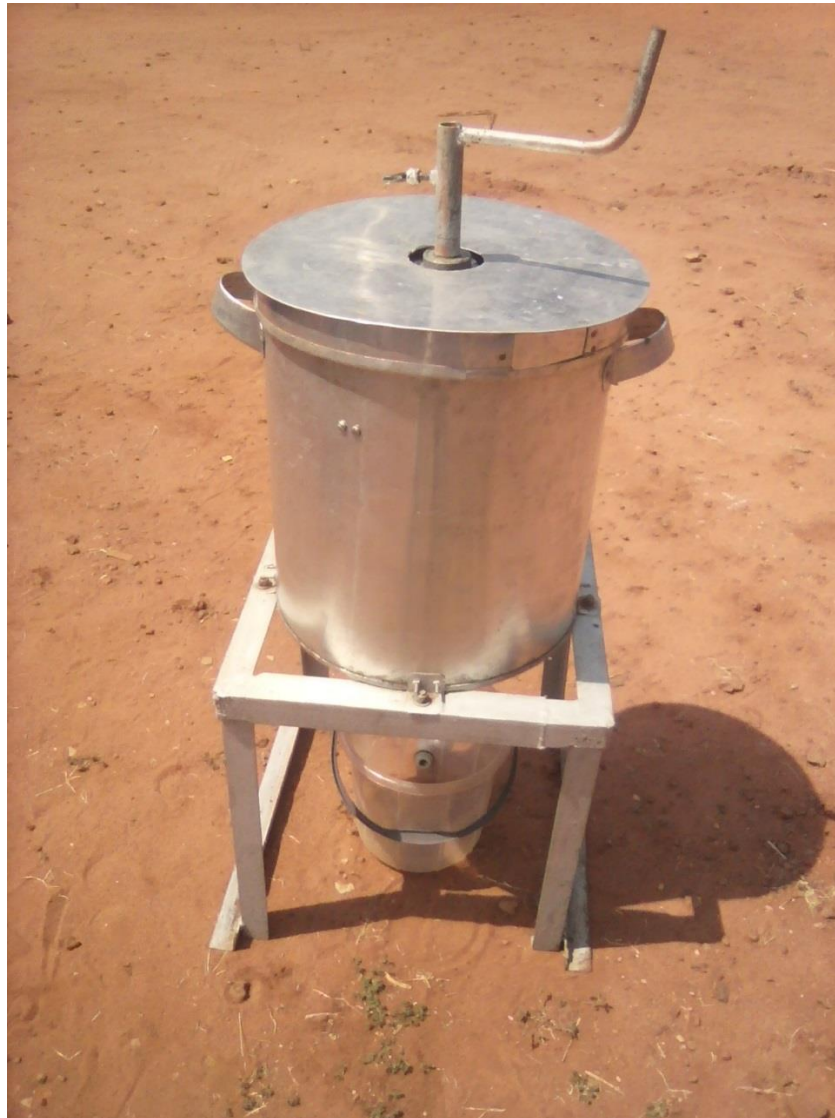
Fig. 3 The wet sieving equipment in a full set up position for a sieving operation
