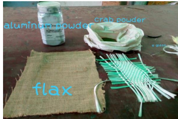
Figure 11) the materials used for the matrix material the flux, E glass, Aluminum powder
