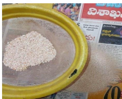
Figure 8) the electrically grinded crab shell powder for filtration
