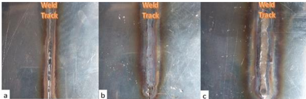
Figure 12 Topographies of the welds under different grain welding conditions: (a) 10A (b) 30A (c) optimized condition
