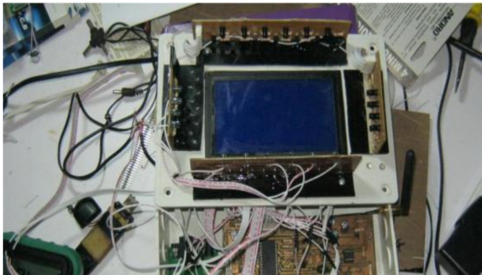
Figure 7: Mounting the LCD screen on within the touchless sensor arrays
