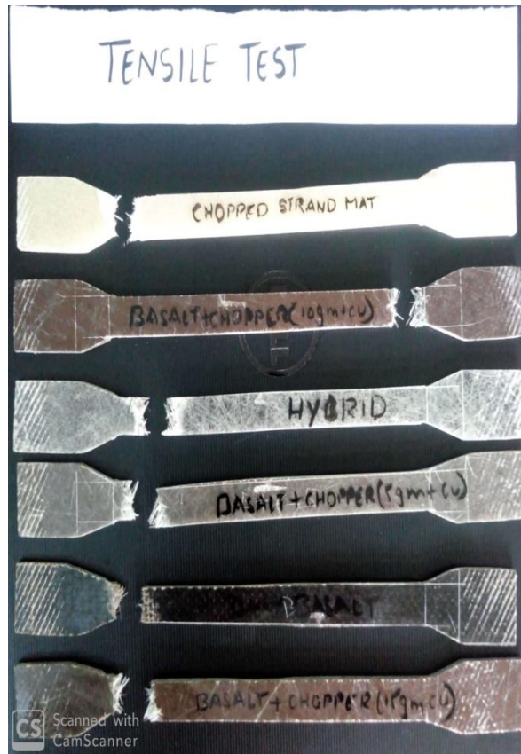
Figure7 Specimens after failure
