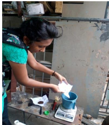
Figure 3 Mixing of copper powder in resin
