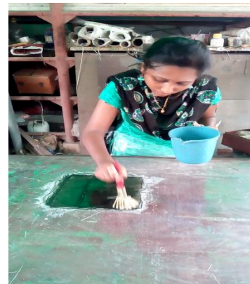
Figure 4 Applying of filler material on the fibre mat
