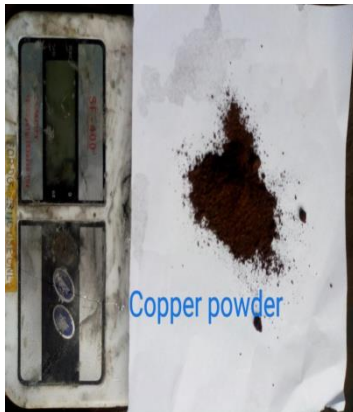
Figure 2 Weighing of copper powder used for hybrid material
