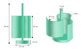
**Figure A**Physical model of the three-bucket Savonius Rotor
