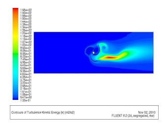
**Figure 18**Variation of turbulence kinetic energy along upstream and downstream side of Savonius rotor (At 16.88% overlap)
