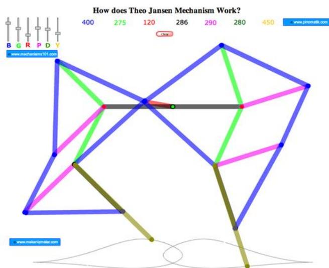
**Figure 1** Theo Jansen linkage mechanism
