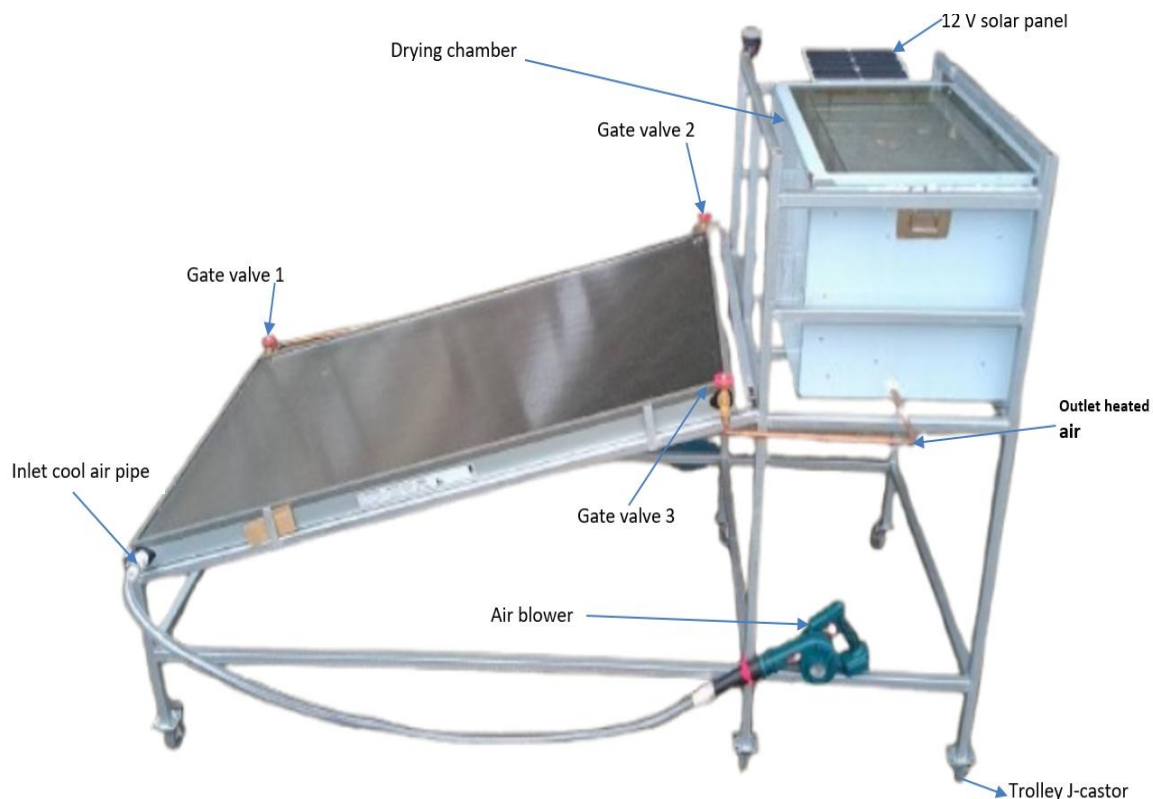
Figure 4: The Indirect Active Solar Heating dryer under no loading condition
