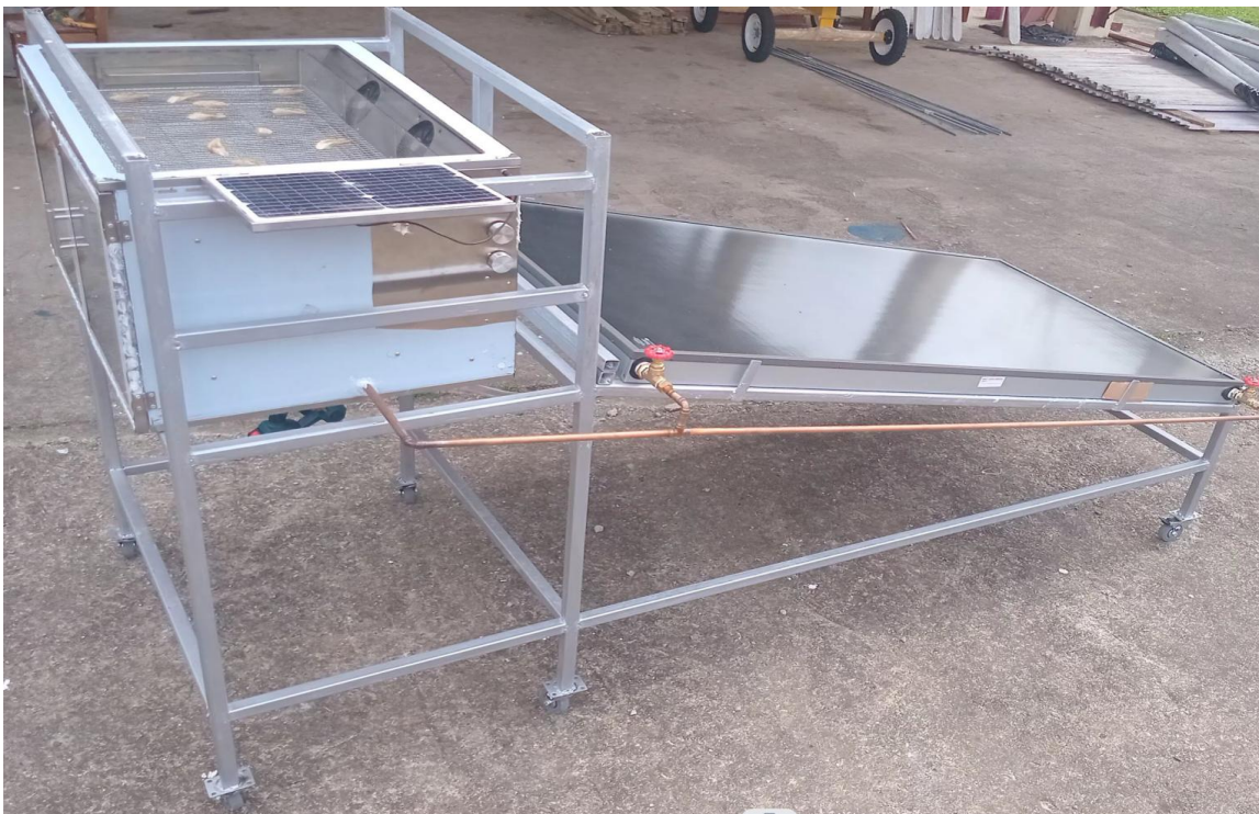
Figure 5: The Indirect Active Solar Heating dryer under loading conditions
